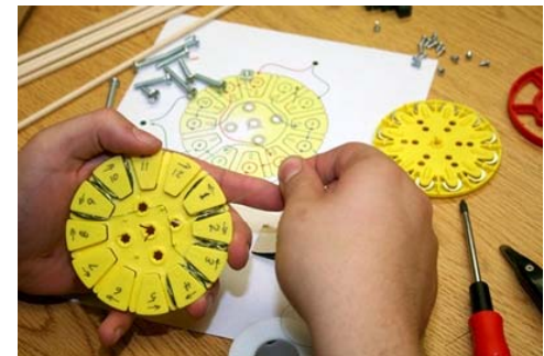
A student creating an Alternator from TeacherGeek components.
