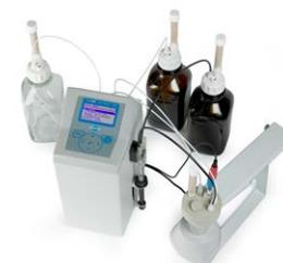
The Karl Fischer TitraLab automatic analyzer is specifically designed for fast volumetric moisture titration, providing the perfect solution to routine measurements. Automatic reagent addition; Solvent addition/waste disposal. Burette volumes available include 1x5mL glass syringe. Languages include Spanish, English, French, and Italian.
