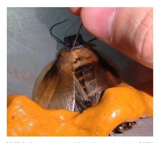
3.3) With fine forceps (or tweezers) carefully insert the center electrode 1mm (0.039") into the hole you just made. It helps to straighten the tip of the electrode as much as possible before inserting.
