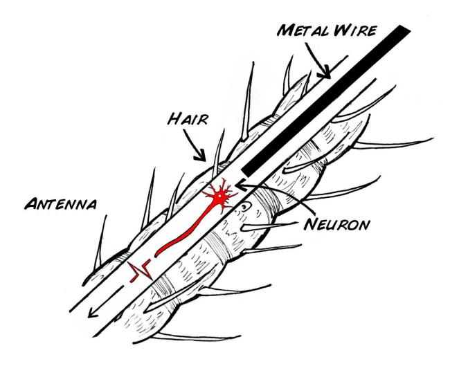
These "spikes" will then travel to the roach's ganglia and stimulate the natural sensio-motor reactions. This is how you can control your cockroach's movement. Basically stated: if we stimulate the neurons on the right antenna, the cockroach will react by turning left. If we stimulate the neurons on the left antenna, the cockroach will turn right.
