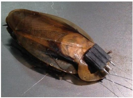
2.5) Place the roach back into the ice for 1-2 minutes to ensure it is continually anesthetize (or until no response to stimuli is observed).
