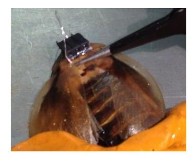
If you need to secure it further, add an extra small bead of super glue above the insertion point, then replace the wing to it's resting place. After the glue has set, a light tug can test if the ground electrode is secure.
