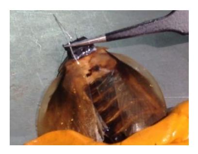
3.4) Using a toothpick apply a small bead of the super glue to the electrode just above where it enters the tissue.
