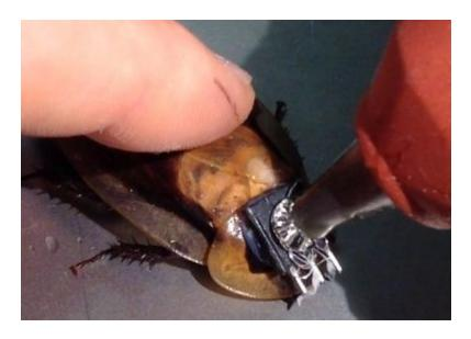
6.4) Quickly after applying the hot glue, use your "floured" flat edge and smush down hot glue. The purpose of the flour is to prevent the hot glue from sticking to your smushing tool.
