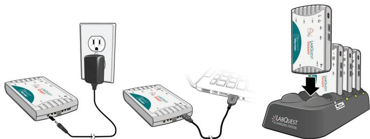
The Charging LED,
