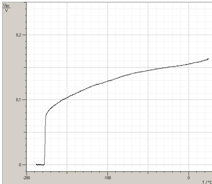
Fig. 4: Voltage drop at the transition temperature of approximately  $-180^{\circ}\text{C}$ .
