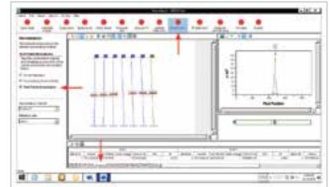
**Figure 4.** Total protein normalization in AzureSpot. TPN is a normalization option in the AzureSpot software. Simply select the normalization method and indicate which channel contains the total protein reference data.
