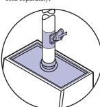
Work surface, on some models, is included. Select the model that fits your application and installation. On some models, a solid epoxy dished work surface is included. Other models include a Type 304 stainless steel work surface. Models without a work
