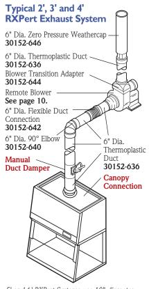
5' and 6' RXPert Systems use 10" diameter ductwork (not shown). Ductwork components noted in **red bold** are included with each RXPert Single Filtered Balance System.
