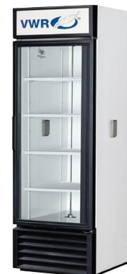
All units feature a natural refrigerant that is environmentally friendly. The R290 hydrocarbon refrigerant emits zero (0) ozone depletion potential (ODP), and three (3) global warming potential (GWP). Units are supplied standard with the LAE temperature control, which offers exterior digital display and alarm function.
