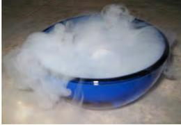
Dry ice is  $-77^{\circ}\text{C}$ . In many cases, the end-user may not really need such a low temperature. It is used because it is relatively inexpensive, easy to purchase or even make, and completely non-toxic. Despite the benefits of dry ice, a chiller can be advantageous in the long run as it replaces the need to keep dry ice (or its components) on hand or continually purchase it.
