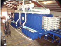
Hydrocooling is the process of chilling food, such as fruits and vegetables, in order to stop the process of ripening without freezing, which destroys the composition of the food. The shelf life of foods is also extended by hydrocooling.
