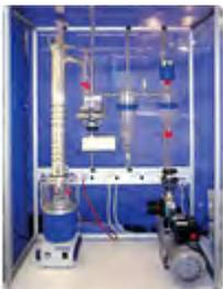
Distillation is a technique for separating components of a mixture on the basis of differing boiling points. The mixture is heated, vaporizing some of the components. The vapor is collected and condensed to isolate the components with the lowest boiling points.
