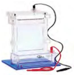
Electrophoresis is the rate of movement of each component in a colloid suspension (gel) while under the influence of an electrical field. Substances, especially proteins, are separated and molecular size is analyzed. It is very important that the gel chamber is maintained at the proper operating temperature to ensure that heat energy from the electrical current passing through the gel will not damage the gel. Therefore, refrigerated circulators can be used to cool the buffer within the chamber.
