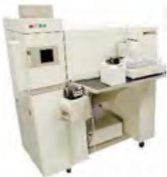
Inductively Coupled Plasma (ICP) is a type of plasma source where electromagnetic induction produces electric currents which supply energy. ICP is utilized in many different applications for elemental analysis. utilized in many different applications for elemental analysis. One technique involves using ICP for the detection of trace metals in environmental samples.
