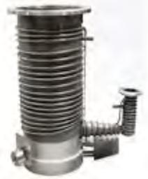
A diffusion pump is basically a stainless steel chamber containing vertically stacked cone-shaped jet assemblies. At the base of the chamber is a pool of a specialized type of oil having a low vapor pressure. The oil is heated to boiling by an electric heater beneath the floor of the chamber. The vaporized oil moves upward and is expelled through the jets in the various assemblies to pump out vapor molecules to create a high vacuum.
