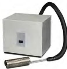
Solvent traps are designed to capture solvent vapors from extractions, often to comply with any safety requirements. For example, a possible source of contamination is oil from a pump that uses the oil either as working fluid or lubricant. Therefore, a solvent trap can be put at the start of the pump to collect any vapors.
