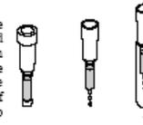
2. Using a new pipette, carefully and gently load 250  $\mu$ l of the “+” supernatant onto the top of the column. Hold the pipette tip against the side of the column wall, just above the upper surface of the matrix and let the supernatant drip down the side of the column wall. Examine the column using a UV light. Note your observations. After it stops dripping transfer the column to collection tube 2.
