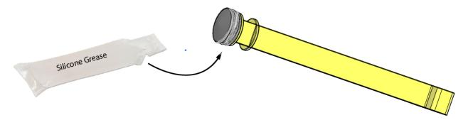
A small amount of silicone grease will lubricate many plungers.
