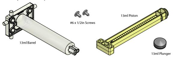
The following steps show construction of a 13ml cylinder. The same process can be used to create 4.5ml cylinders.
