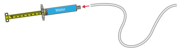
**Step #4**Push the cylinder piston completely in to fill the tubing with water.
