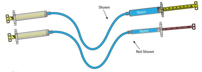
**Step #1**Assemble the required cylinders and cut the appropriate length of tubing.
