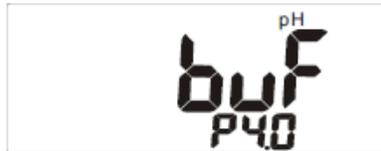
3. Press **←** to enter P4.1. The default “NIST” will flash on the LCD and P4.1 will appear on the lower portion of the display. If you use NIST buffers, press **←** to confirm and the meter returns to P4.0.
