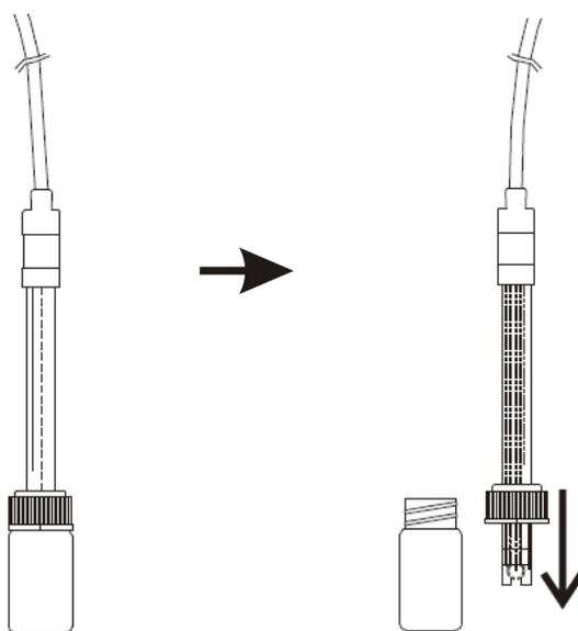
1. Rotate the bottle to remove the bottle from the probe. Pull down the cover and remove it from the probe.
