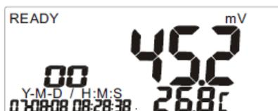
4. Press **MODE** to switch between mV and pH.
