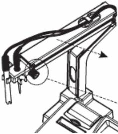
The holder can hold up to 4 probes. The wire of the probe can be fixed to the arm.
