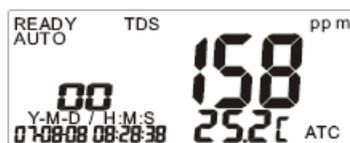
6. Press **MODE** to switch between TDS and CON/SALT.
