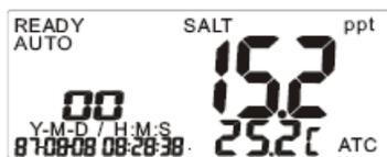
6. Press **MODE** to switch between SALT and CON/TDS.
