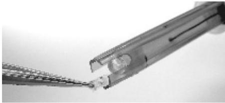
2. Cut the clogged fiber and expose the new portion.
