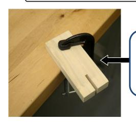
Clamp the slider block to the edge of a sturdy table.
