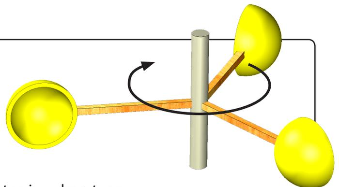
A cup anemometer is a drag-type vertical axis wind turbine
