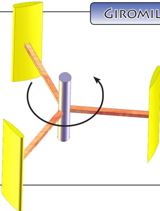
The giromill is typically powered by two or three vertical aerofoils attached to the central mast by horizontal supports. Giromill turbines work well in turbulent wind conditions and are an affordable option where a standard horizontal axis windmill type turbine is unsuitable.
