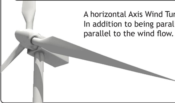
A horizontal Axis Wind Turbine is the most common wind turbine design. In addition to being parallel to the ground, the axis of blade rotation is parallel to the wind flow.
