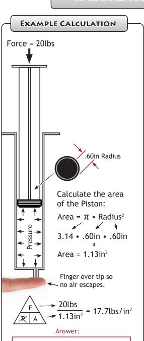
The Air Pressure inside the syringe chamber = 17.7psi
