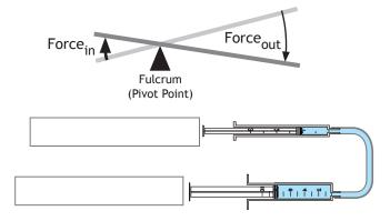
**52.** Label the Force<sub>in</sub> and Force<sub>out</sub> on the cylinders below to show a mechanical advantage similar to the lever.
