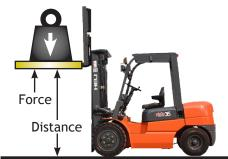
Forklifts use hydraulics to perform work (moving loads)
