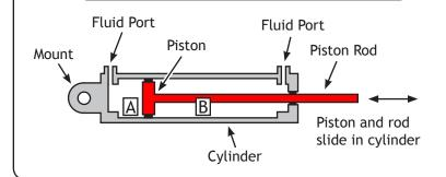
Chambers A and B are sealed, so fluid can only enter or exit through the ports. Pressure in a chamber creates a force on the piston.
