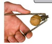
Mechanical Advantage is the relationship between the work going in to a system, and work coming out of a system.
