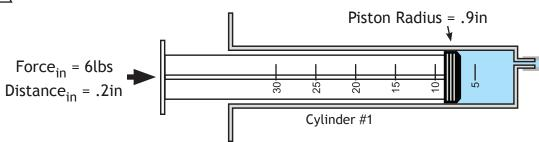
Piston Force Developed From Fluid Pressure Over Piston Area:
