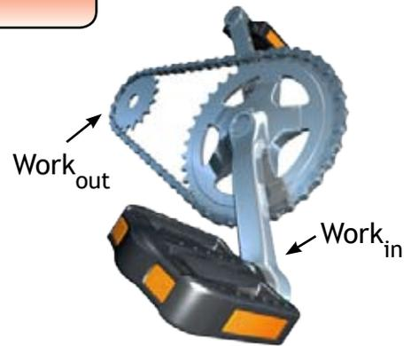
$$\text{Mechanical Advantage} = \frac{\text{Distance}_{\text{in}}}{\text{Distance}_{\text{out}}} = \frac{\text{Force}_{\text{out}}}{\text{Force}_{\text{in}}}$$
