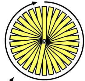
A wheel works like a lever revolving around an axis.
