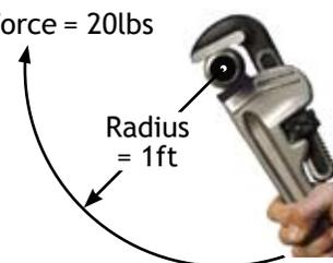
What is the torque applied to the pipe?
