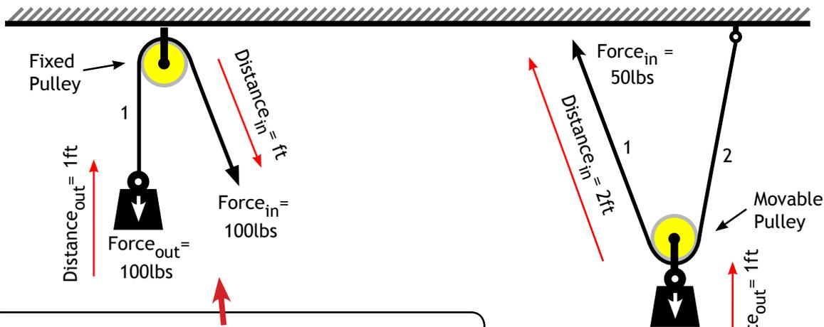
1 Line Supporting the Load = Mechanical Advantage of 1 (no mechanical advantage)
