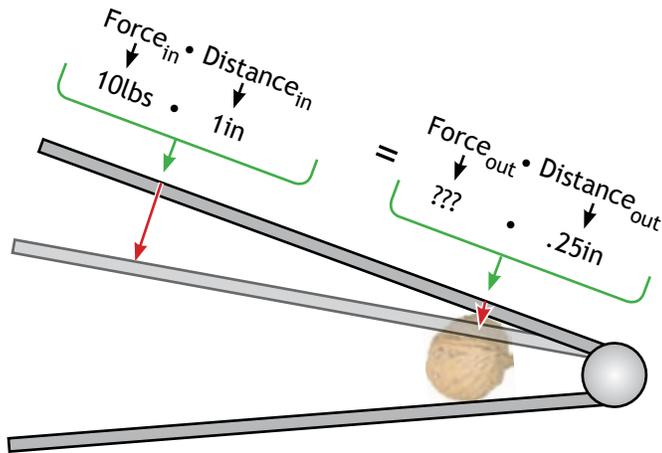
① Mechanical Advantage =  $\frac{\text{Distance}_{in}}{\text{Distance}_{out}} = \frac{\text{Force}_{out}}{\text{Force}_{in}}$
