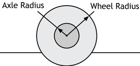
$$\frac{\text{Torque}_{\text{out}}}{\text{Torque}_{\text{in}}} = \frac{\text{Input Radius}}{\text{Output Radius}}$$
