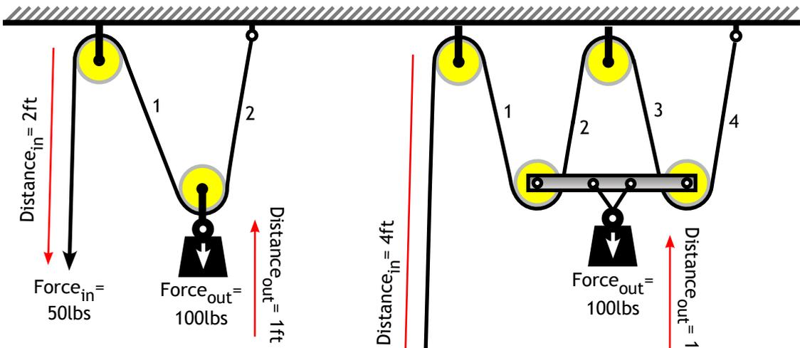
2 Lines Supporting the Load = Mechanical Advantage of 2
