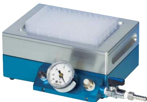
Pall's multi-well vacuum manifold is designed to perfectly fit SBS-conforming filter plates. The spacer block has been optimized to reduce the space between the receiver plate and the filter plate during vacuum filtration. The adapter collar holds filter plates tightly to receiver plates for centrifugation.
