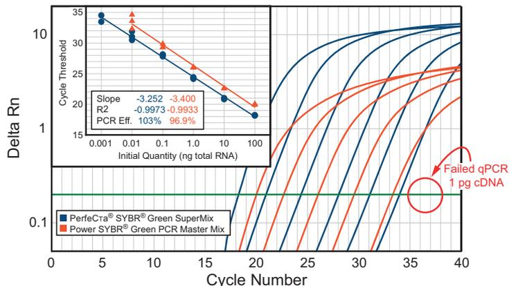
PKCA Target: qScript™ cDNA from HeLa cell total RNA, Log-fold serial dilutions (100ng to 0.1pg) in triplicate, run on ABI 7500.
