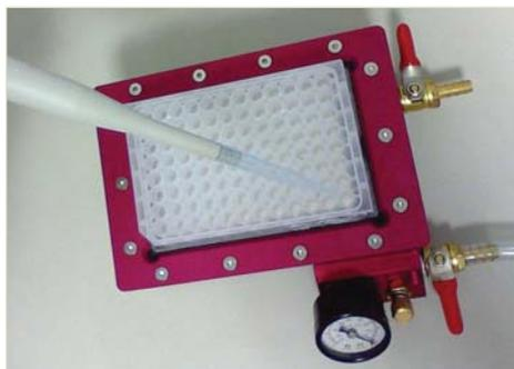
The IBI vacuum manifold for 96-Well plates is made of anodized aluminum for long life and easy cleaning. Fits most standard 96-Well extraction and collection plates. Thin upper body of manifold prevents well-to-well cross-contamination. Easily assembled, it can be used for plasmid purification, genomic DNA extraction, viral DNA & RNA isolation, and total RNA isolation and PCR/Gel purification. IBI 96-Well purification kits are designed for optimal use with the 96-Well manifold.
