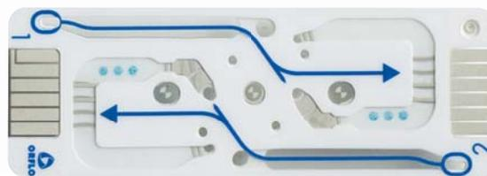
Precision microfluidic cassette keeps your sample safely contained. No cleaning, no maintenance.
