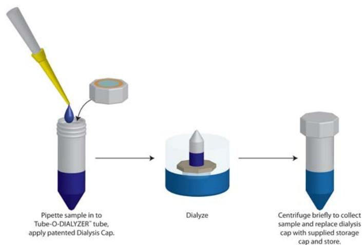
G-Biosciences manufactures a unique dialysis device that allows efficient dialysis and ensures 100% sample recovery, even if precipitation occurs. The Tube-O-DIALYZER micro dialysis system is designed for small sample volumes of 20µL to 2.5mL. The patented tube design of Tube-O-DIALYZER permits easy sample loading, sample handling and manipulation, without the use of specialized loading devices, costly syringes, or hazardous needles.
