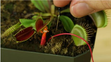
6. Plug the yellow RCA jack with black and red electrode clips into the Plant SpikerBox. Attach the Red clip to the red recording wire and the black clip to the black grounding wire.
