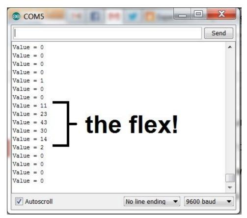
If this does not work, you may need to adjust your spikershield's potentiometer (pictured below - depending on the model number of your shield the potentiometer may be located somewhere else on the board). Give it a slight rotation clockwise to increase the gain and test it again in the serial monitor. Repeat this process until you receive results in the serial monitor similar to the ones pictured above.
