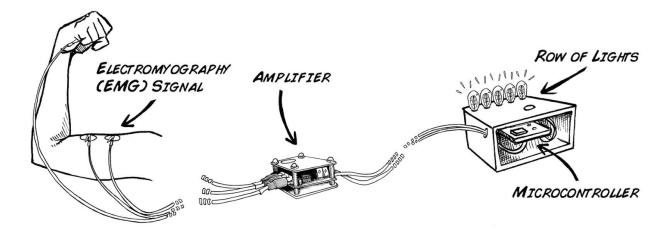
Importantly, the Arduino converts the EMG signal from an analog (continuously varying) into a digital one (broken into discrete "numbers"), making analysis and instructions on what to do with the signal much easier.
