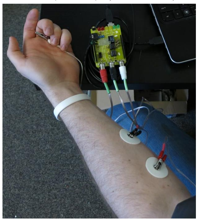
3. Open the Arduino serial monitor from the IDE to check the values. If you get larger values when you flex your muscles, and values near zero when you don't, then everything is working ok! If not, make sure all cables are connected correctly and nothing is loose. You may find connecting a portable speaker to the
