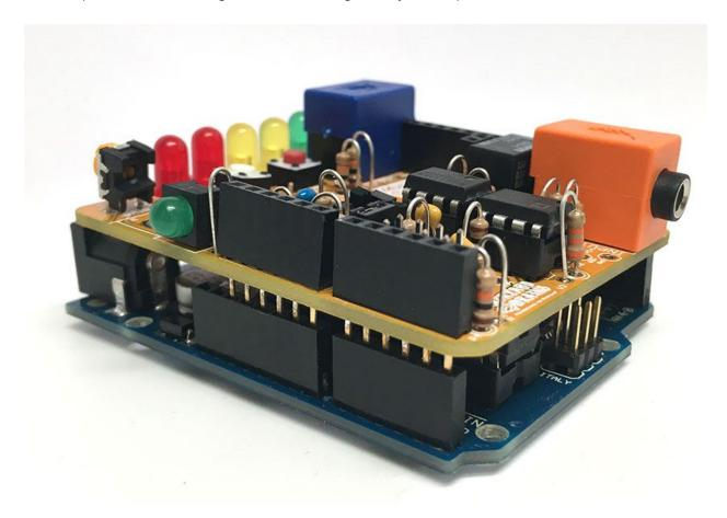
2. Download our serial\_test2014.ino sketch (also mentioned above) and upload it to your arduino. Then connect the orange electrode cable wire from the Muscle SpikerShield to some electrodes on your arms. Hook the two red clips onto your arm and place the black one on the back of your wrist. You can also plug in a speaker to hear your muscle activity alongside the visual outputs!
