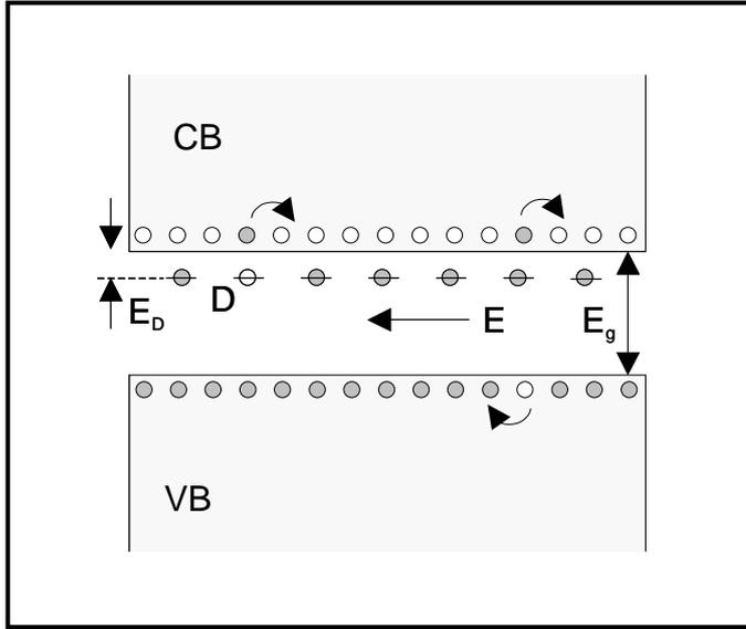
Fig. 2: Simplified diagram of extrinsic (left) and intrinsic conduction (right) under influence of an electric field E: Incorporating of dopants (donors D) into the crystal lattice creates negative charge carriers (electrons) in the conduction band (CB). With increasing temperature the thermal energy of valence electrons increases allowing them to breach the energy gap  $E_g$  into the conduction band (CB) leaving a vacancy called hole in the VB.
