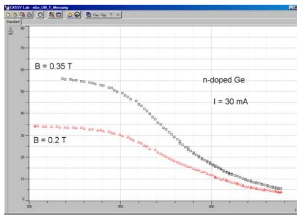
Fig. 6: Hall voltage  $U_H$  as function of the temperature  $T$  for  $I = 30 \text{ mA}$  and different magnetic fields  $B$ .
