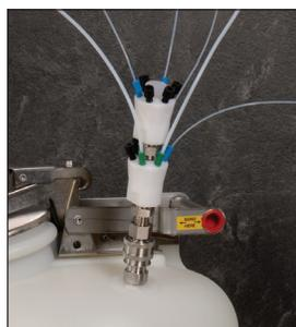
Manifold no. 94000-348 with stacker no. 94000-352 and tubing connector package nos. 94000-354 and 94000-356.
