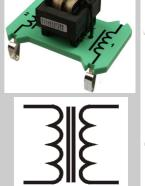
coils with a 'core' linking the magnetic field of one coil to the other.
