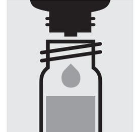
Add 3 drops of **Mg-2K**, close the cell with the screw cap and mix.
