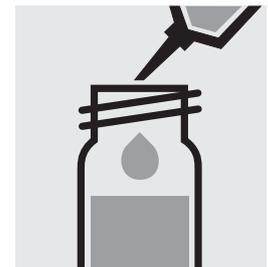
Add 5.0 ml of **Zn-6** (Cat. No. 106146, Isobutyl-methylketone) with pipette and close the test tube with the screw cap.
