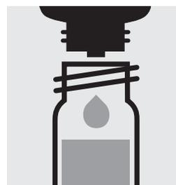
Add 2 drops of **T-2K**, close the cell with the screw cap.
