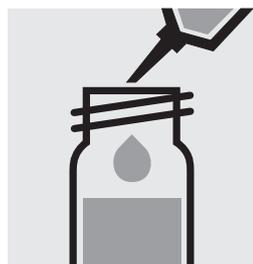
Add 0.80 ml of **B-3** with pipette, close with the screw cap, and mix.
