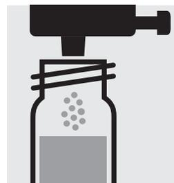
Add 1 dose of **P-2K** using the blue dosing cap, close the cell with the screw cap.
