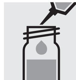
Add 0.25 ml of **Al-2K** with pipette, close with the screw cap, and mix.
