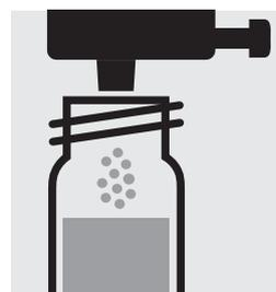
Add 1 dose of **Cr-2K** using the blue dose-metering cap, close the reaction cell with the screw cap.
