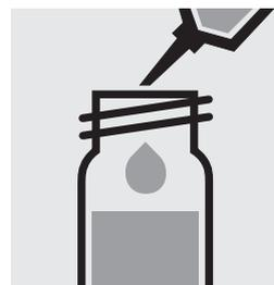
Add 0.50 ml of **reagent 2** with pipette, close the cell with the screw cap, and mix.
