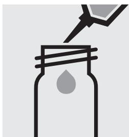
Pipette 4.0 ml of **AC-1** into a round cell.
