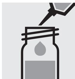
Add 0.50 ml of **AC-2** with pipette, close the cell with the screw cap, and mix.
