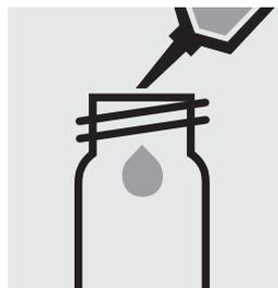
Pipette 10 ml of the sample into a test tube (Flat-bottomed tubes, Cat.No. 114902).
