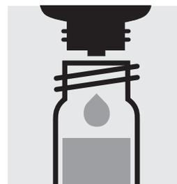
Add 15 drops of **B-5**, close with the screw cap, and mix.
