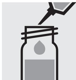
Add 5.0 ml of the sample with pipette, close the cell with the screw cap, and mix.
