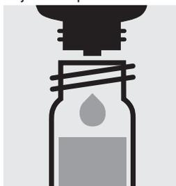
Add 5 drops of **Zn-3K**, close the cell with the screw cap, and mix.
