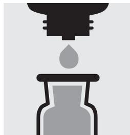
Add 5 drops of **BOD-1K** and then 10 drops of **BOD-2K**, close bubble-free, and mix for approx. 10 seconds.
