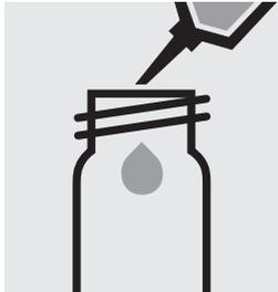
Pipette 4.0 ml of the sample into an empty round cell (Empty cells, Cat.No. 114724).
