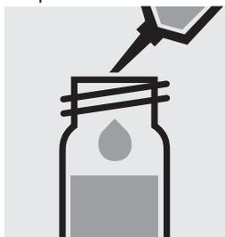
Add 7.0 ml of distilled water with pipette to the second reaction cell, close with the screw cap, and mix. (Blank)
