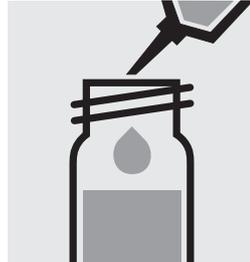
Add 1.0 ml of **Mg-1K** with pipette, close the cell with the screw cap, and mix.
