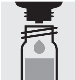
Add 5 drops of **P-2K**, close the cell with the screw cap, and mix.
