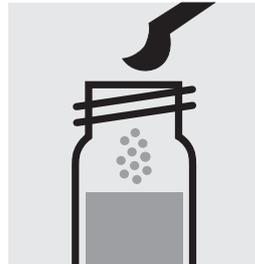
Add approx. 1.5 g of **aluminium chloride hexahydrate extra pure** (Cat.No. 101084), close the cell with the screw cap.
