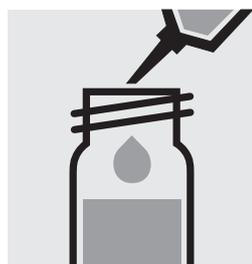
Add 1.0 ml of **Ca-1K** with pipette, close the cell with the screw cap, and mix.
