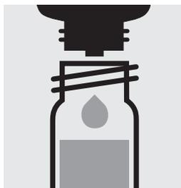
Add 4 drops of **pH-1**, close the cell with the screw cap, and mix.
