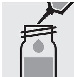
Add 1.0 ml of **NO<sub>3</sub>-1K** with pipette, close the cell with the screw cap, and mix. **Caution, cell becomes hot!**
