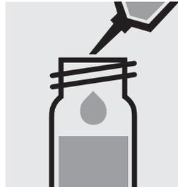
Add 8.0 ml of the sample with pipette and close with the screw cap.
