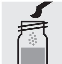
Add 1 level grey micro-spoon each of **SO<sub>3</sub>-1K** into two reaction cells, close with the screw cap.
