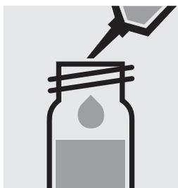
Pipette 3.0 ml of stirred sample into a reaction cell.
