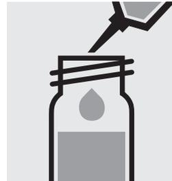
Add very slowly 1.5 ml of the sample with pipette, close the cell with the screw cap, and mix **briefly**. **Caution, cell becomes hot!**
