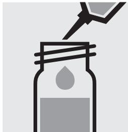
**Carefully** pipette 3.0 ml of the **depleted sample** into a reaction cell, close tightly with the screw cap, and mix vigorously. **Caution, the cell becomes hot!**
