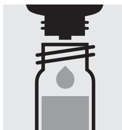
Add 4 drops of SO<sub>4</sub>-4 to the filtrate, close the test tube with the screw cap, and mix.
