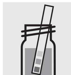
Check the pH, specified range: pH 1.5 – 3.5. If required, add dilute sulfuric acid drop by drop to adjust the pH.
