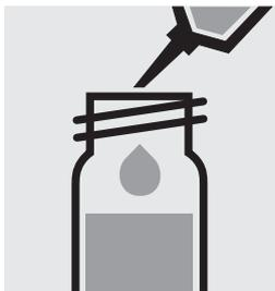
Add 1.0 ml of **OA-3** with pipette, close the cell with the screw cap, and mix.
