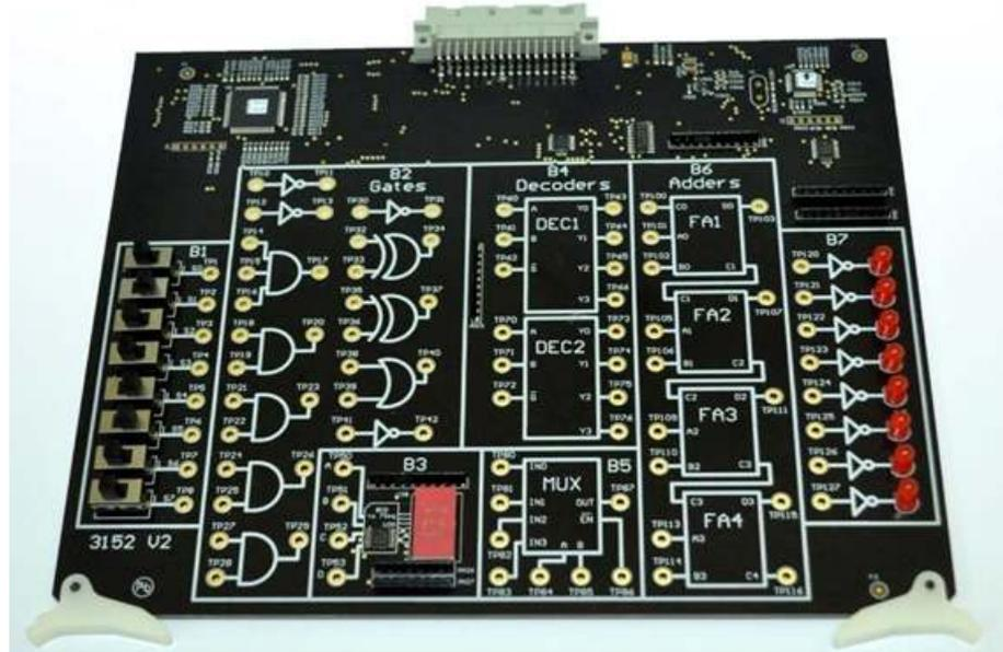
The EB-3152 Multiplexers, Decoders and Adders board is a comprehensive instructional module designed to introduce the student to the basic concepts of various decoders, creating a logic function with a decoder, multiplexers and their use in implementing logic functions and binary arithmetic implementation to students in high schools, technical schools and colleges.
