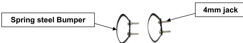
**3.3.2 Release Bumper accessory:** This accessory is used with Inclined plane to hold Car at height. It fits in the 4mm socket at the end of the track. The lever holds the Car with the Elastic Bumper. When lever is pressed the Car is released from the End of the track as shown below.
