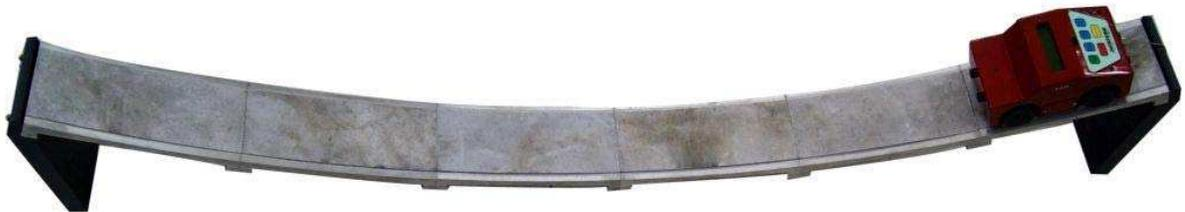
Switch ON the Car by pressing **ON/OFF** key. Place Car on the track. Start the timer using **START/STOP** key on Car or **IR REMOTE**. Release and allow the Car to move in to and fro motion on the Potential Well Track to record motion data. After few movements stop the recording by pressing **START/STOP** key on Car or **IR REMOTE**. Data collected can be reviewed through key pad or can be loaded in software for analysis by selecting menu **Data>Data Load from Car** as explained in section 4.3.
