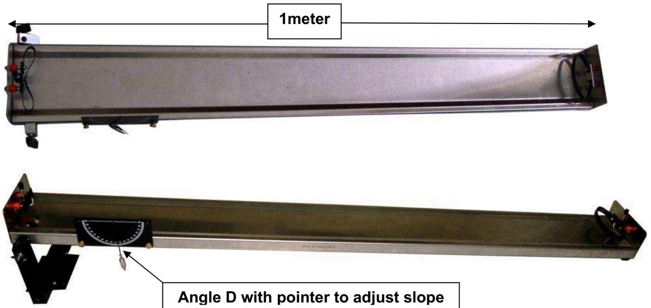
It is Stainless Steel Track with an arrangement of mounting bumper accessory with 4mm jack fitted on both sides of track. Track is provided with Scale and marker to adjust an angle to perform inclined plane experiments. Stainless Steel material helps in decreasing the frictional losses while performing experiments. This track can be used to perform Linear Motion on Horizontal and Inclined plane experiments as well as Elastic and Inelastic collision experiments.
