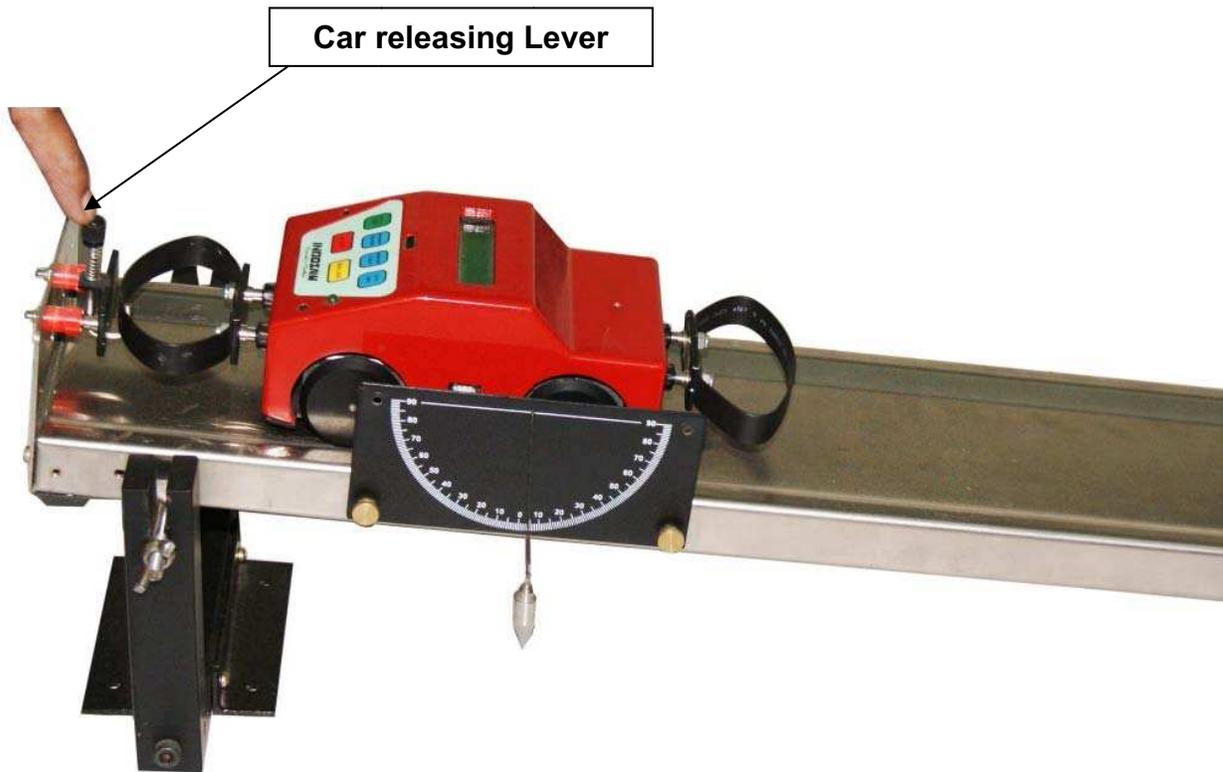
**3.3.3 Striker Bumper accessory :** This accessory is used on Track for striking or providing Initial Momentum to Car. The Spring Strip is compressed to hold in the lever as shown below. When lever is pressed the Spring gets released to strike the object placed near it with a force which provides initial Momentum.
