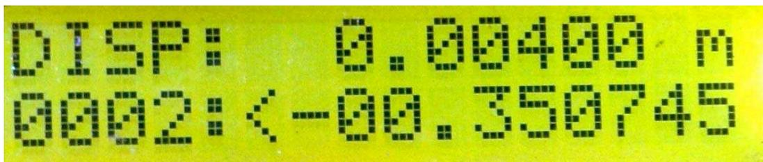
The displacement is displayed in linear vector form considering the start of recording as zero Displacement. With every press of the Memory Review key the reading number is incremented and correspondingly displayed.
