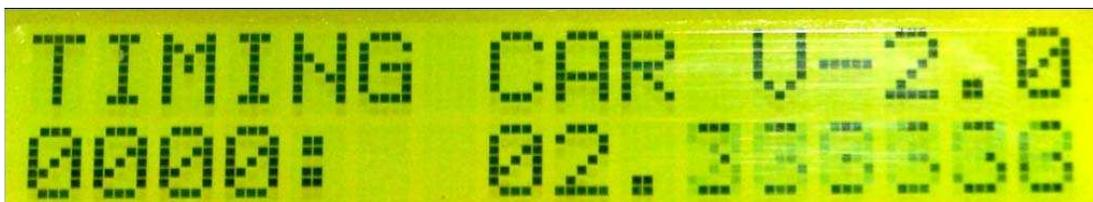
When Car is moved on track or plane, every 2 Millimeter of Displacement, the number reading increments on the left half of 2<sup>nd</sup> line on LCD. The maximum four digit reading reaches to 9999 after which the recording stops. Same START/STOP key is used to STOP the timer if counter has not reached to 9999 reading. When timer is stopped the display is shown below.
