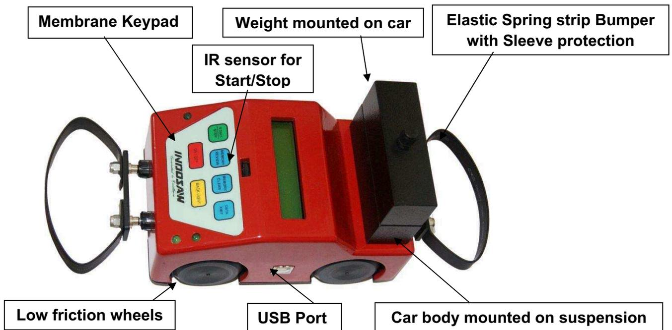
The Car is low friction device and body is mounted on suspension at its wheels. The car has provision for mounting front and rear bumper accessories and weights. It has a 9v replaceable battery and USB port. It has an IR detector for remote timer on/off. The LEDs display the motion status. Duracell 9v battery is recommended.
