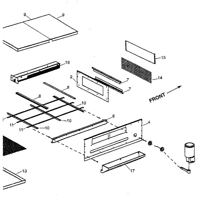
Ref. 22 10-24 Nuts go on the inside -Use Ref. Nos. 19, 21 and 22 fasteners in top holes (use the longer 3/4 screw in top hole at each corner)
