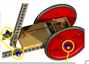
Slide-Stop Material keeps components with "loose" reamed holes from sliding back and forth on dowels. Turn the screw into both components.
