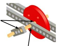
The link strip holes that the dowel needs to rotate in were reamed to make them larger
