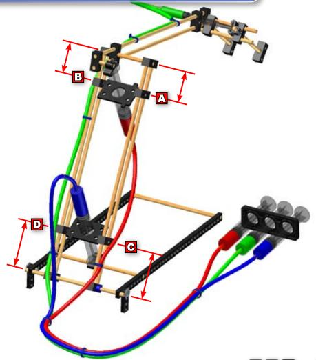
Sliding the perpendicular adaptors attached to the syringe mounts ( $\triangle$ ,  $\square$ ,  $\square$  and  $\square$ ) changes the travel/mechanical advantage of the arm.
