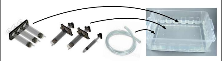
Food coloring can be added to better see the fluid flow through the hydraulic system.
