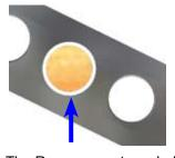
The Reamer creates a hole that is larger than the dowel.
