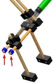
2 Add slide stop material to keep the gripper from opening too far and getting stuck.
