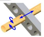
The dowel moves freely in the loose fitting hole.
